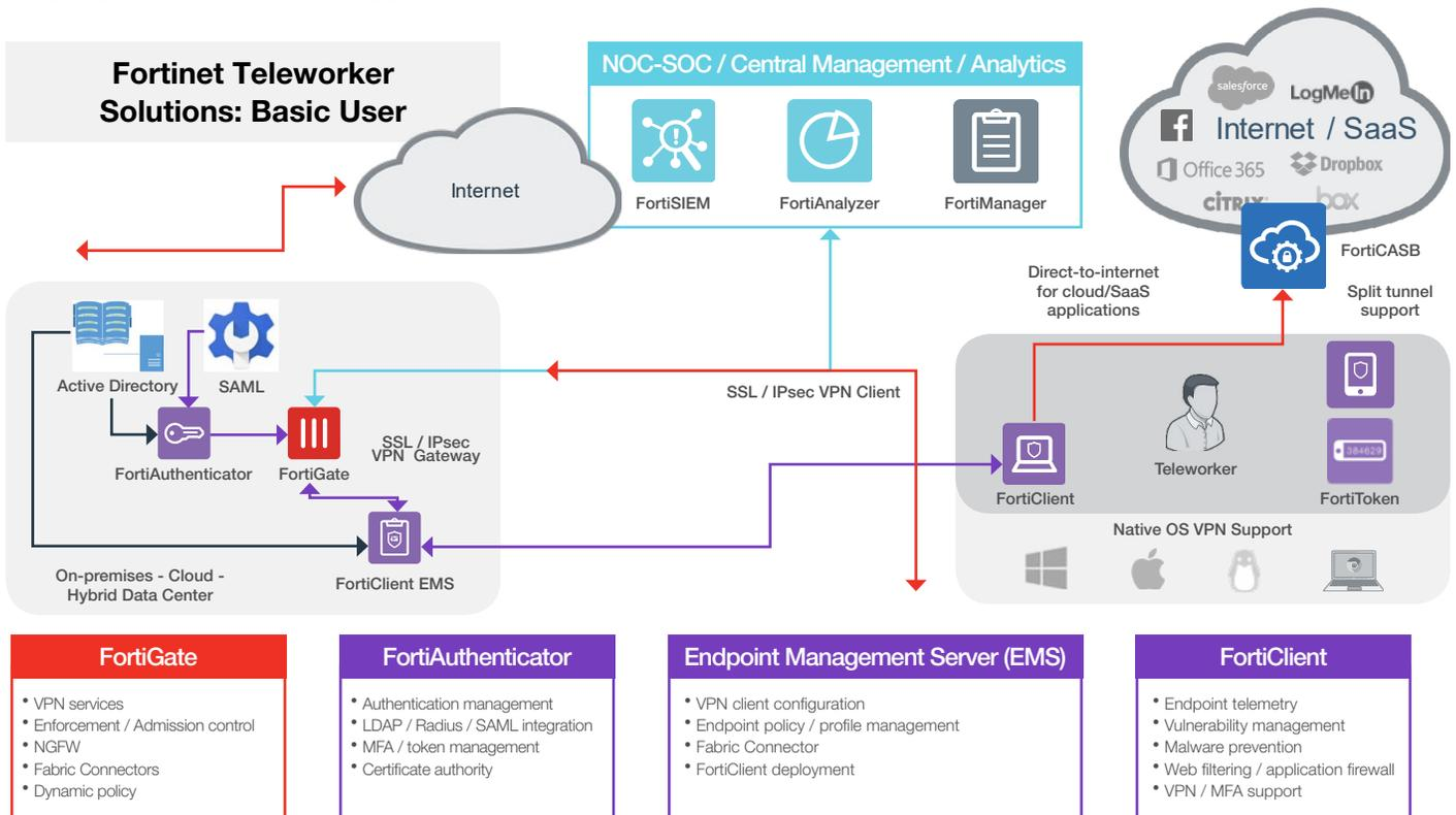
Figure 1: Notional Fortinet solution deployment for basic teleworker.
