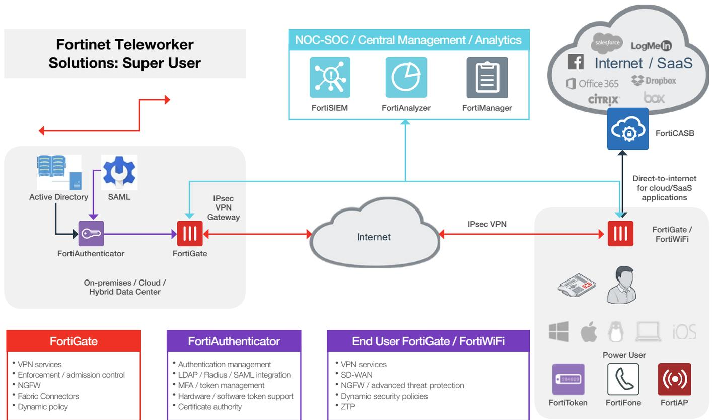
Figure 3: Notional Fortinet solution deployment for super user.
